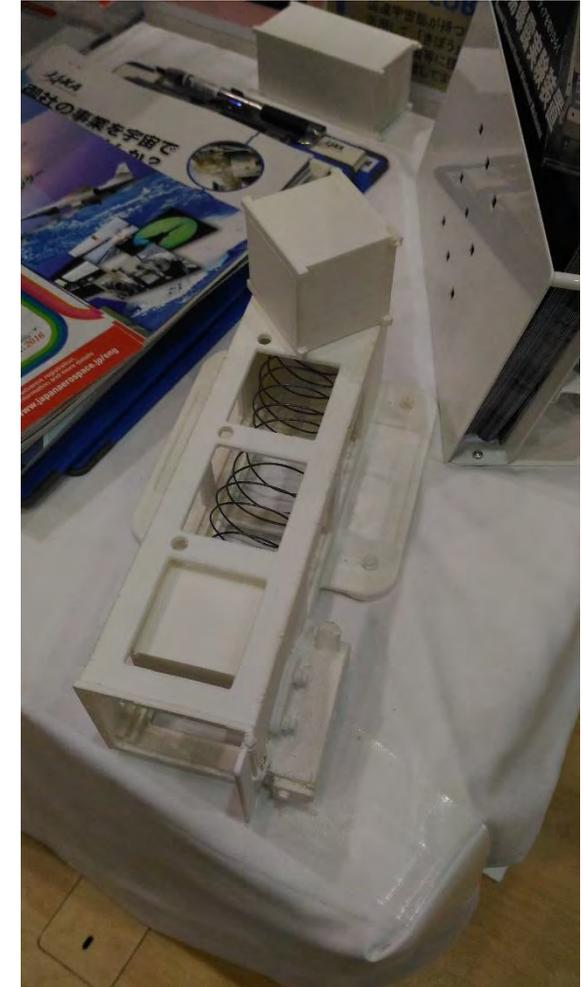
Half-size 3D print model of JEM Small Satellite Orbital Deployer (J-SSOD); BIRDS CubeSat will use the J-SSOD for its deployment from ISS
