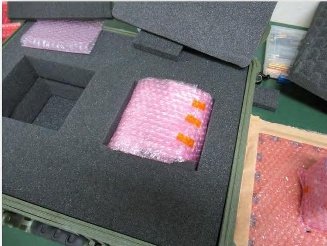
Each CubeSat was carefully wrapped with multiple layers of bubble wrap covering all sides a day before place inside Pelican box.
