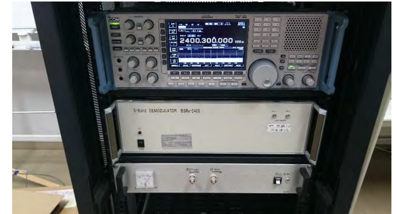
IC-R9500 (Receiver for HORYU-IV S-band) with demodulator. This is the biggest amateur radio machine in KyuTech.
