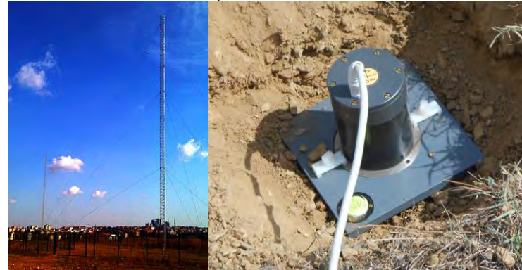
HF Ionosonde VIPIR in ITU –on left- and the fluxgate magnetometer –on right- installed in Bozcaada by SWL members.
