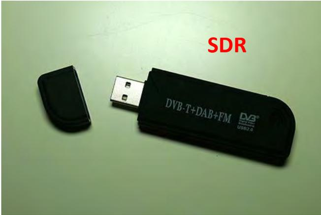
This is an SDR (software defined radio) dongle, which you can easily buy from Amazon. Most are in the \$15-\$30 range because the core component is essentially the same (a chip called **R820T/2**).
