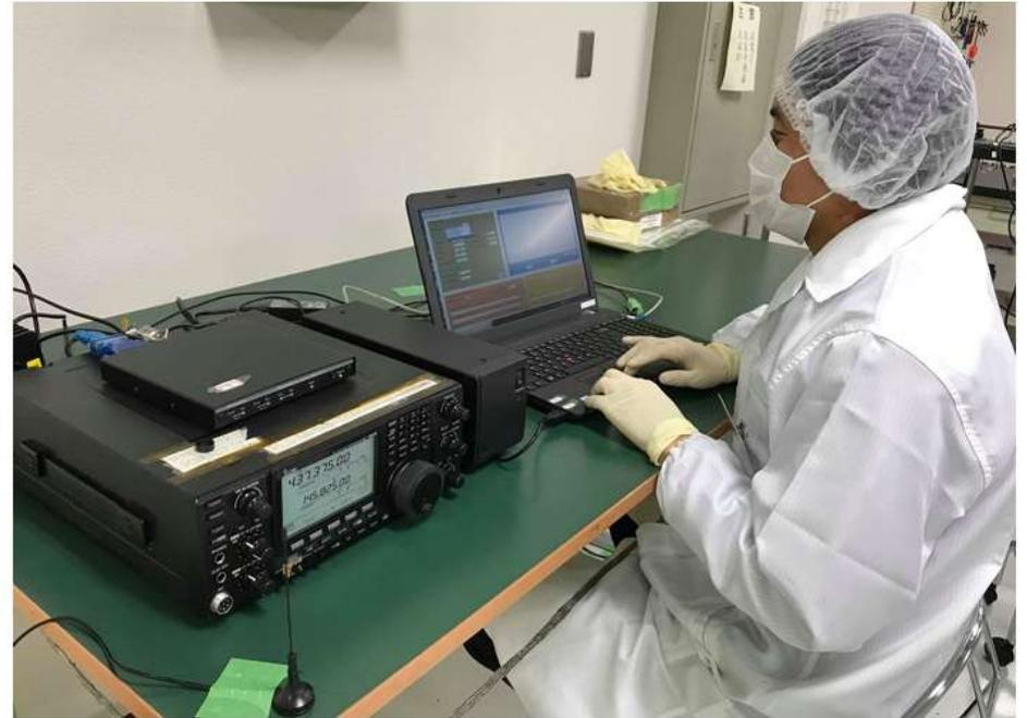
Verifying that software initialization and loading were properly done by downloading and checking the data at the ground station
