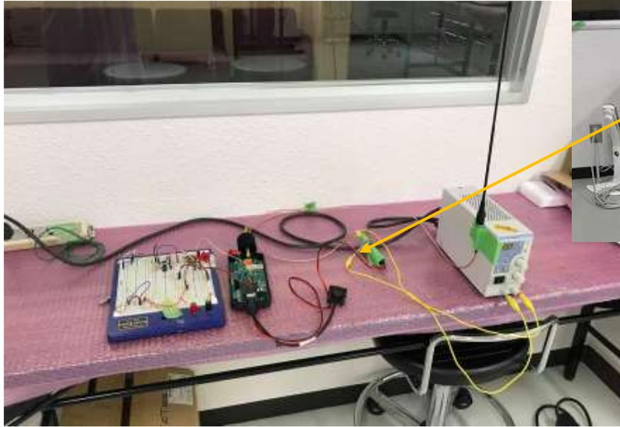
Dummy Ground Sensor Terminal to test functionality with the Store-and-Forward payload
