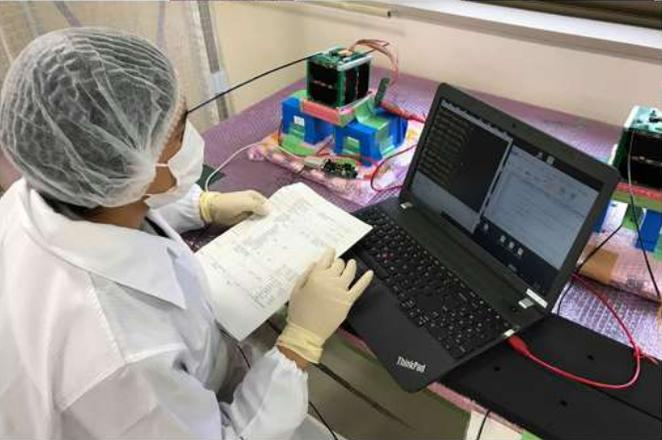
Initialization of flash memories and loading the programs to respective onboard microcontrollers
