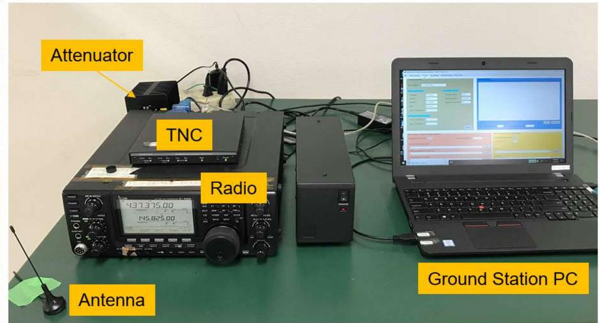
Above left is the preliminary end-to-end test setup. Using a solar array simulator (instead of a typical power supply), we also checked the satellite power budget and operation under several sunlight and eclipse cycles. Above right is the ground station setup used to communicate with the satellite.
