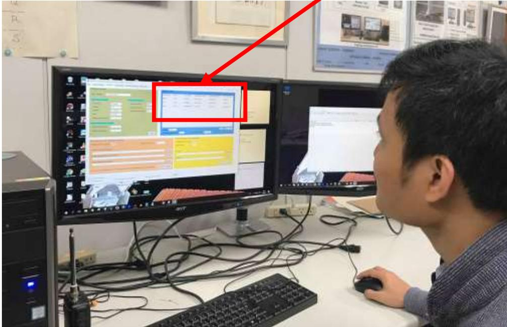
Ground station software was used to immediately process and display the results of operation such as CW beacon, latest satellite housekeeping telemetry, log, image file database, etc.
