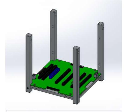
Pic: Backplane mounted with the structure frame
