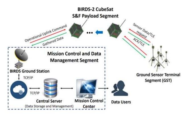
System architecture of BIRDS-2 S&F CubeSat constellation-based remote data collection system (RDCS)
