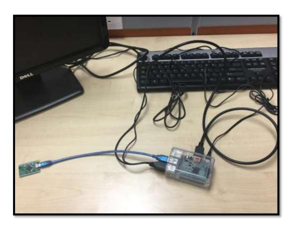
Shows the connection of Raspberry Pi with T3 mini tracker
