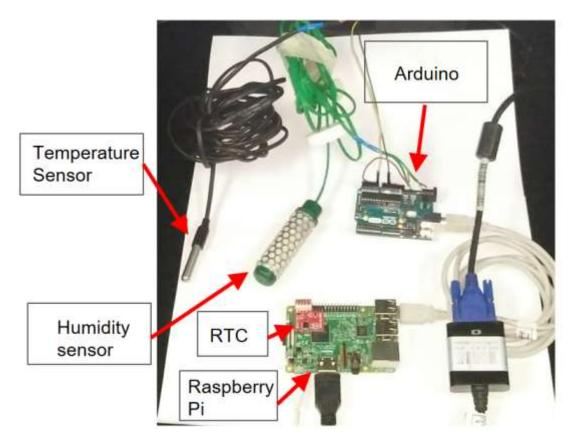
Photos of the initial GST development setup. Programming of the Control and Communication Unit (Raspberry Pi 3) has been focused to implementing the communication protocol, data logging and satellite pass prediction.
