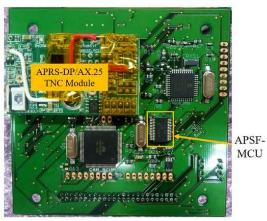
APRS-DP/AX.25 TNC module soldered on the mission board (back side), which also houses other parts of S&F payload and other mission payloads and subsystems
