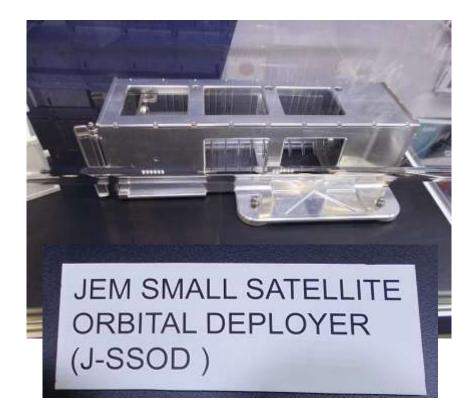
All BIRDS satellites are deployed into space by the ISS using this special "deployer".
