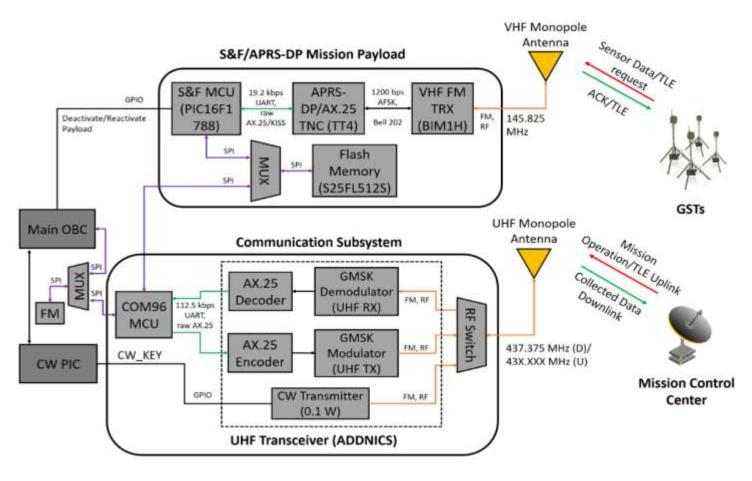
Block diagram of onboard S&F Mission Payload Segment and CubeSat's Communication Subsystem
