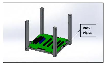
*Fig. 5 (Above): (STEP-3) Assembly of base frame with side rails and the installation of backplane*
