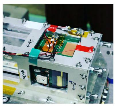
Fig. 4: EM Ready for Vibration Testing
