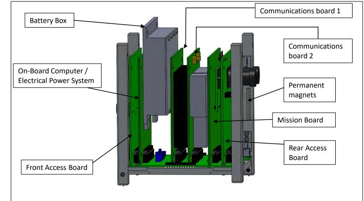
*Fig. 6 (above): (STEP-4) Attaching the magnets on rails and all the boards including battery box*
