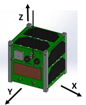
Fig. 1: CubeSat axis definition
