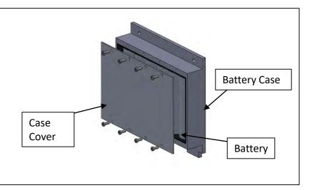
Fig. 3: (STEP-1) Preparation of battery box
