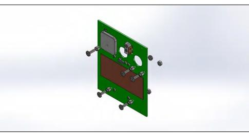
Fig. 4: (STEP-2) Preparation of +Y panel for circuit burner for monopole antenna and holding it before deployment
