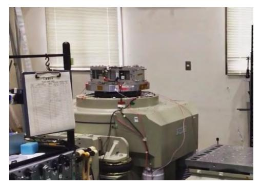
Fig. 5: BIRDS-2 EM under vibration test
