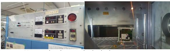
Vacuum chamber---to check whether antenna will work under vacuum condition or not
