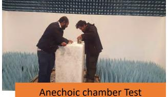
UHF/VHF antenna test for BIRDS satellite demonstrate the test to measure the radiation pattern, gain and VSWR from the antenna attached with the satellite.
