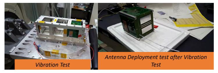
**Vibration Test-** To demonstrate the ability of the satellite antenna system; specially deployment mechanism to meet qualification requirements under vibration conditions which simulate the prediction for flight.
