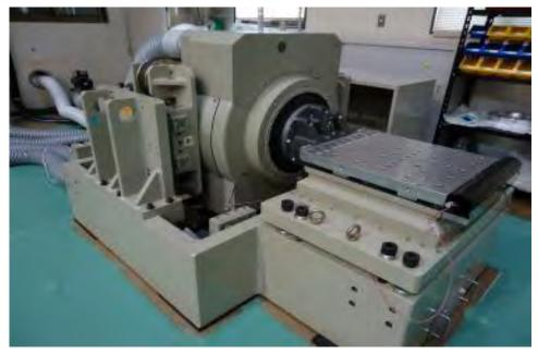
Vibration Testing Machine, Center for Nanosatellite Testing, Kyutech
