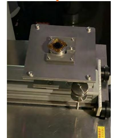
Attaching the sample holder to the sample stage in the EB machine
