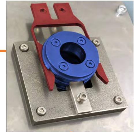
Optical window for measuring optical properties
