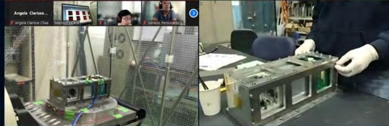
After the antenna deployment tests, vibration test (VT) was performed on the Maya-6 engineering model (EM). The objectives of the VT is to determine the fundamental frequency of the CubeSat structure and to verify the integrity of design workmanship against JAXA's launch qualification requirements.
