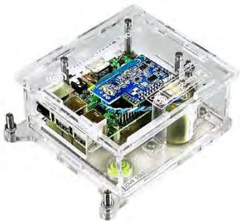
This article is about a low-cost seismometer that can be deployed in any terrain but needs a link to a data center. This link can be an Internet connection – or BIRDS/KITSUNE GST. Below is the link to the manufacturer of Raspberry Shake:
