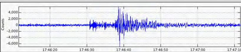
Fig. 2. Station R30E2, located in downtown Pétiön-Ville, produced Haiti’s first Raspberry Shake station recording of a local earthquake on 13 January 2019. This event was not reported by Haiti’s national seismic network, but it was later reported by the Dominican Republic seismic network as an M3.1 event (yellow star in Figure 1) along the Enriquillo–Presqu’île du Sud fault close to the border between Haiti and the Dominican Republic.
