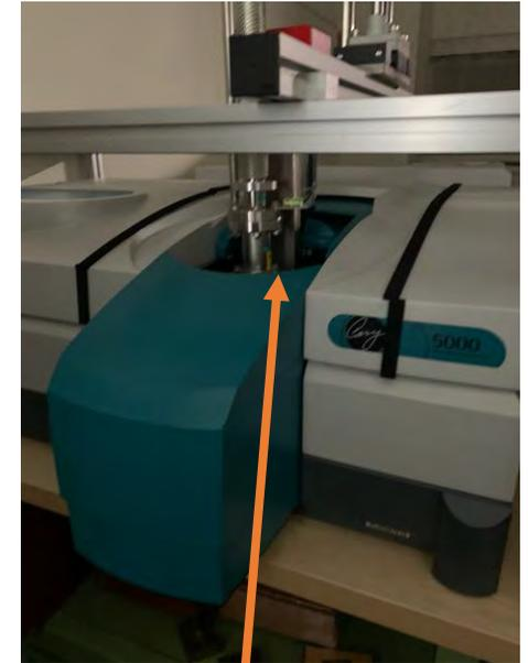
Insertion of the VTV inside the measurement zone
