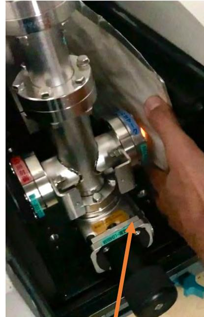
Adjustment of the VTV inside the spectrophotometer
