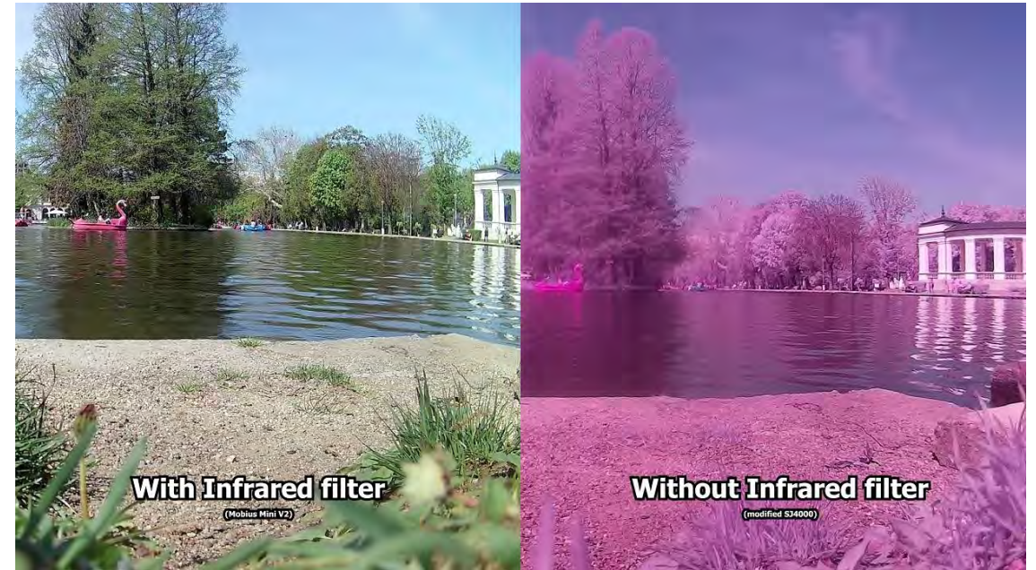
Figure 1: The image difference between camera with and without IR filter.
