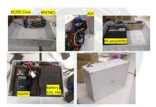
The different components that make up our GST can be compacted into an IP66 Spelsberg Junction box (250x180x90mm).
