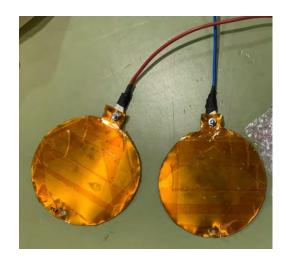
FIRST: In the experiment, a circular copper plate was used as a probe for DLP. This probe was placed in the chamber.
