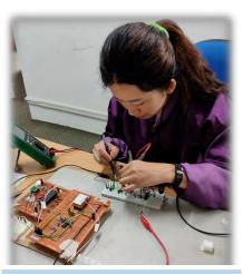
Testing the Power Circuit of the payload on breadboard
