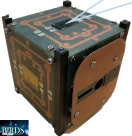
A sun sensor is in the part of attitude control in the satellite that use for measure the incidence angle of sun rays with respect to a reference surface.
