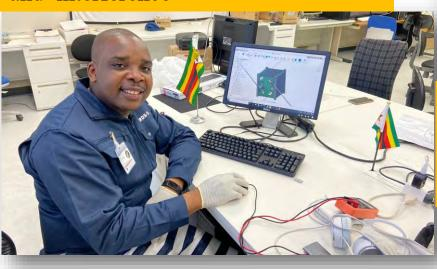
Otani checking a delivered Back Plane Board for functionality, electrical interface and programing of the CPLD and mission Boss Edgar Mujuni from Uganda doing the designing (Schematic and brd) of the Store & forward mission and multispectral mission
