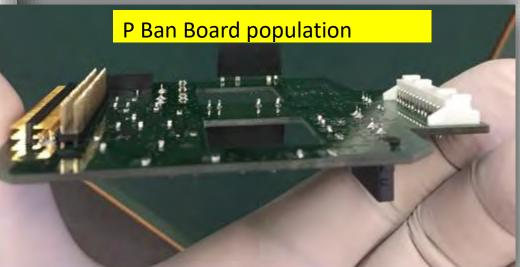
Component interference preventing the mosphets from lying horizontal as in the CAD design
