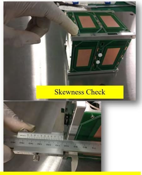
Camera protrusion as per JAXA requirements it should not pass6.5mm from the rail end
