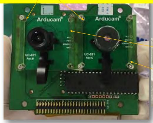
The biggest worry was that will these spacers sustain the random vibration during the space environmental testing. The structure team designed spacers made from PEEK material
