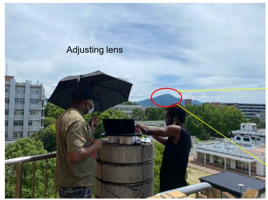
With the camera connected to a display and set to preview mode, we were able to set our lens at its center of focus before applying Araldite.
