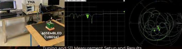
Tuning radiation and pattern measurement for the Hentenna mission was performed. An initial S11 level of -13dB on the tuning frequency was achieved, and the radiation pattern plots for each position are seen on the figures below.
