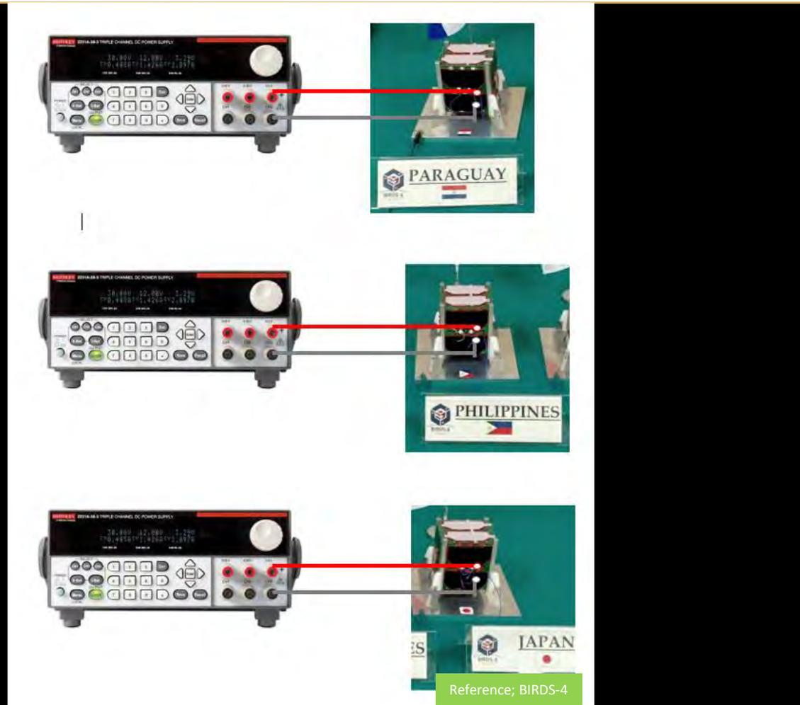
*Satellite battery charging setup. Set voltage output to 5.2 V, 0.8 A.*
