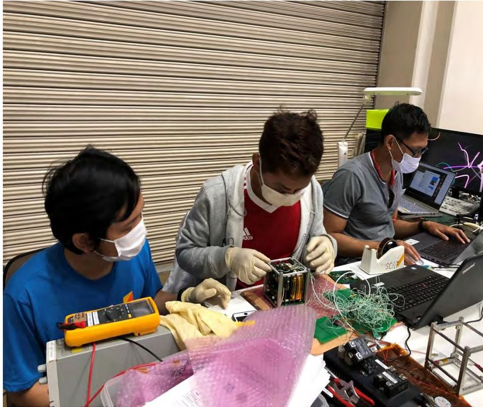
**MAYA3 CubeSat being prepared for thermal vacuum test**
