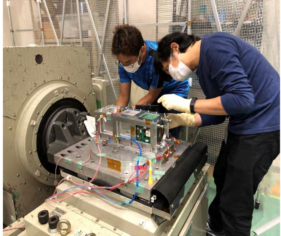
**MAYA3 CubeSat being prepared for vibration test**
