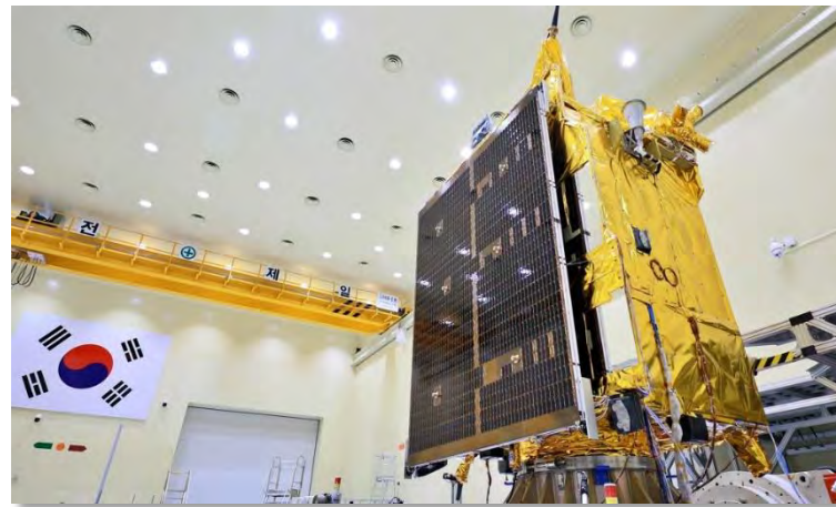
Chollian-2B with its solar panels in folded position. Source: Yonhap
