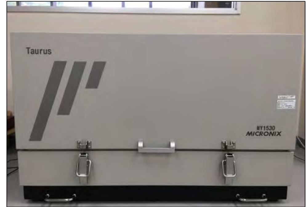
RF shield box at 2F cleanroom of SVBL Building
