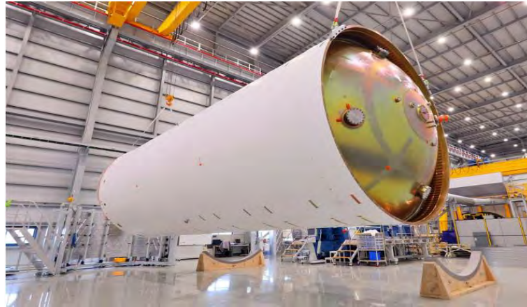
Oxidant tank of the 1 st stage of KSLV-II. Source: KARI
