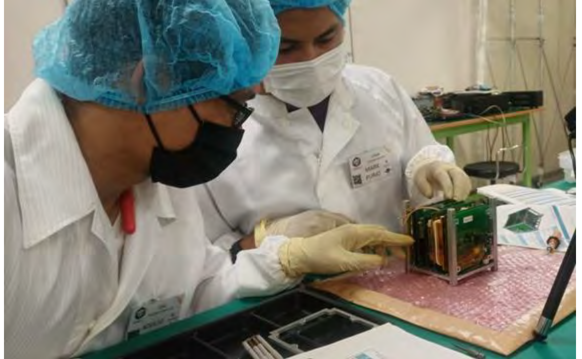
BIRDS-4 members checking the Engineering model of the satellite for functionality testing
