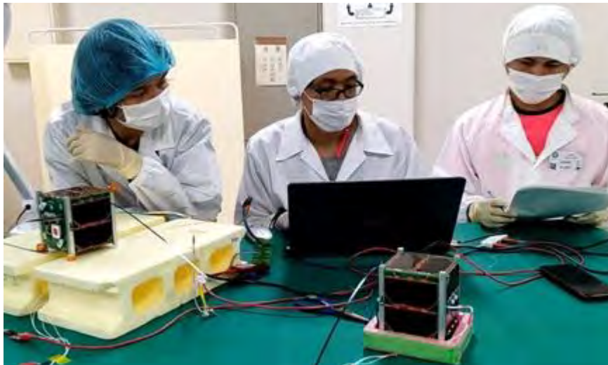
BIRDS-4 members uploading the final flight software for the satellites while following detailed procedures
