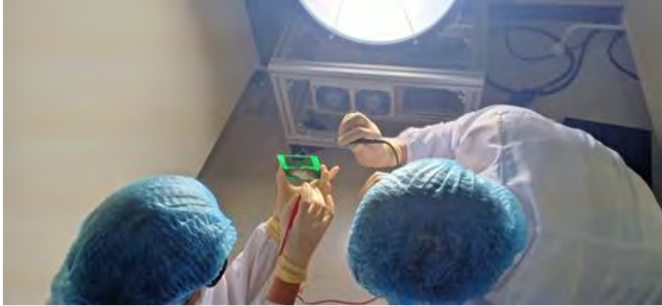
BIRDS-4 members testing final solar panel to ensure power generation for the satellite
