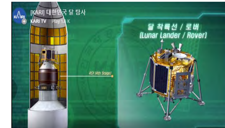
Position of the Lunar Lander/Rover inside of the launch vehicle.
