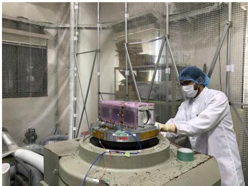
*Yigit is setting up the vibration test*
