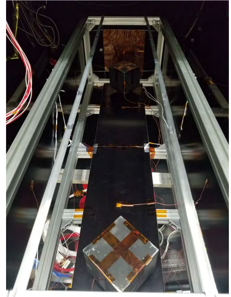
Heaters casing and dummy satellites
