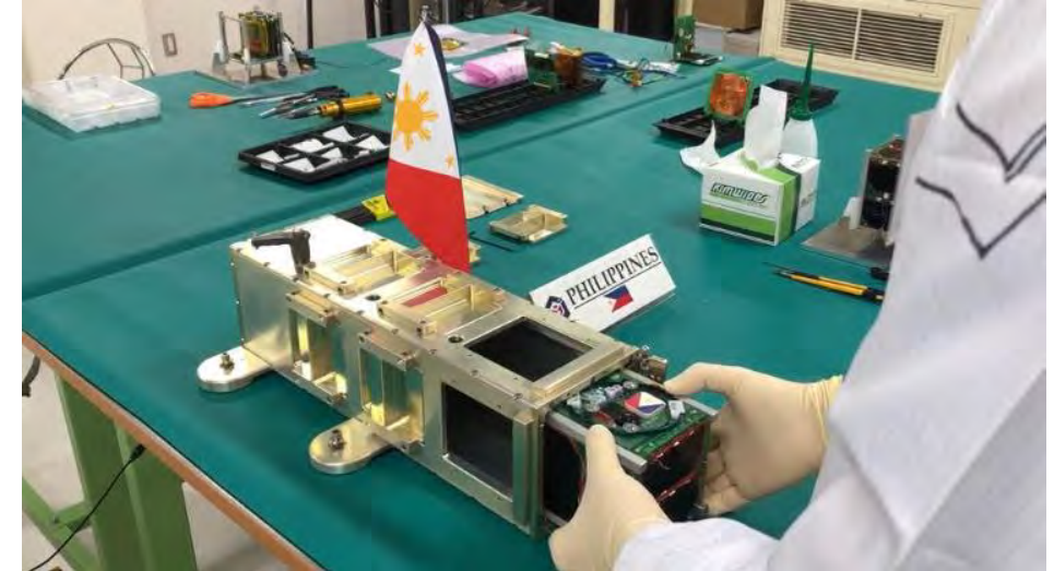
Putting the assembled satellite (Maya-2) inside the pod for fit test and inhibit test of the lever switch inside the rail structure
