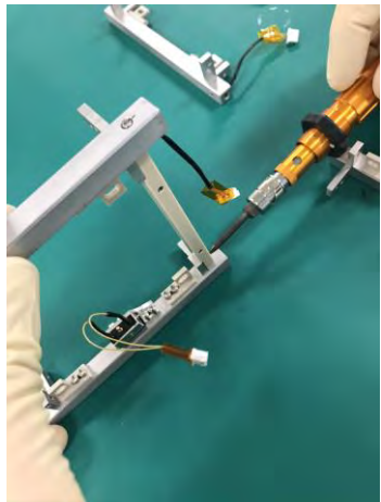
Deployment switches integrated with the structure and back plane board during flight model assembly
